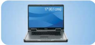
**Intel® Centrino® Mobile Technology** - Intel® Core™ Duo Processor T2500 **Genuine Windows® XP Professional SP2 Edition** Intel® PRO/Wireless 3945 WLAN 802.11a/g Mini PCI Card Intel® 945PM Express Chipset 1GB DDR2 SDRAM 80GB1 Ultra ATA Hard Disk Drive 7200 rpm Integrated Gigabit Network Interface 24X CDRW/DVD3 Combo Drive 17" (43.1 cms) Wide Aspect XGA (1440 x 900 res) TFT Display 3-Year Limited Warranty (Next Business Day On-Site Service<sup>2</sup>)
