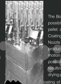
The Bottom Spray method makes it possible to gain excellent results in pellet as well as Powder / Particle Coating. The combination of Spray Nozzle positioned directly in the
