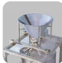
Vibratory Feeding Mechanism For Non Free Flowing Powder.
